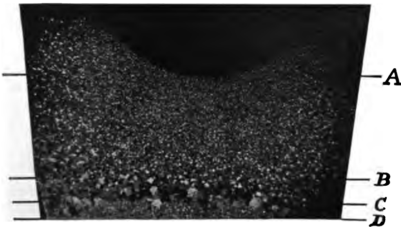
Fig. 2. Steel Section, 0.05 Carbon, Magnified Six Diameters.*
